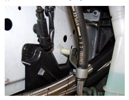
k. Referring to the following image, route the lines through the opening between the passenger side frame rail and the front subframe.
