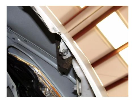
10. Gripping the sides of fascia (circled below) pull the fascia towards you. This part of the fascia snaps in place and will pop loose when a limited amount of force is applied.
