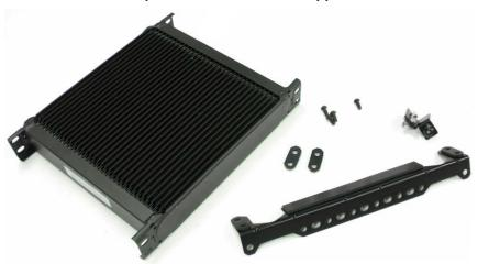
a. Using the Aluminum SETRAB Bracket and it supplied hardware. Attach the bracket to the bottom of the oil cooler (opposite of the end with the fittings). The rotation of the bracket does not matter. The core can be rotated depending on installation preferences. Refer to the image below:
